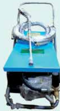
This High Pressure Jet Machine is extremely useful for proper cleaning of CTC/CFM and also used to easily clean in every corner of a narrow place which is not possible for manual cleaning.
